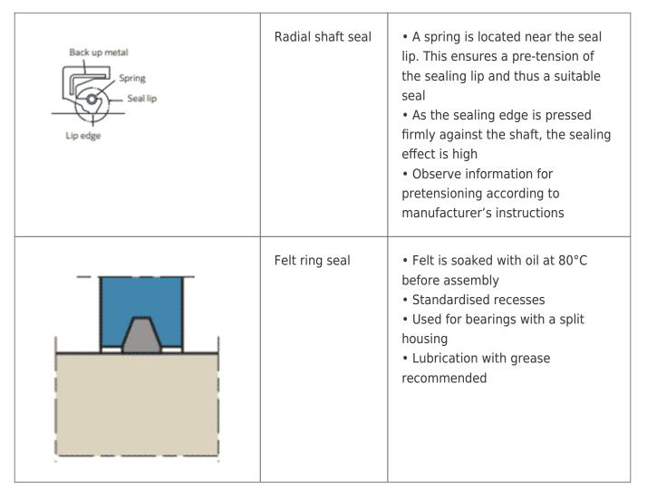
The Z-grease seal, the V-ring seal, the rotary shaft seal and the felt ring seal are all contact seals.
