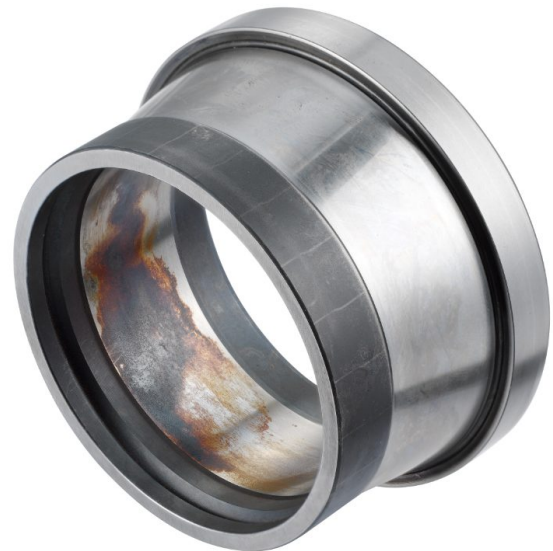
This inner ring is affected by fretting corrosion.
