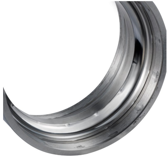
Here, deformations can be seen on a bearing ring.
