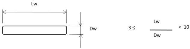
The length to diameter ratio of the rolling elements in needle bearings is shown here.
