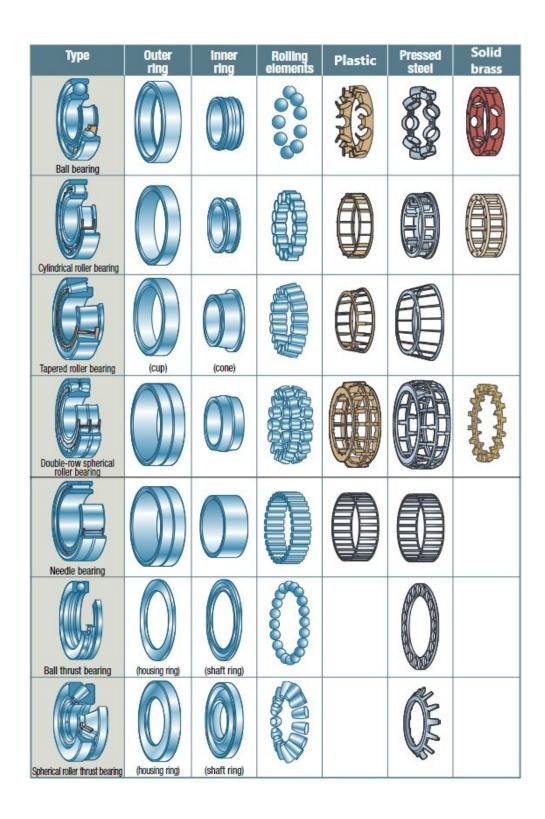
*This table gives you an overview of the most important types of rolling bearings, including their rolling elements and cage designs.*
