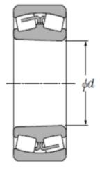
The bearing clearance of spherical roller bearings with a tapered bore can be adjusted more precisely via the displacement path compared to other spherical roller bearings.
