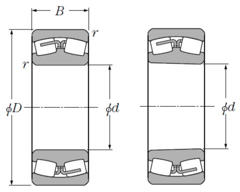
In this technical drawing of a spherical roller bearing, the inner ring, outer ring, both rows of rolling elements and cage are clearly visible.
